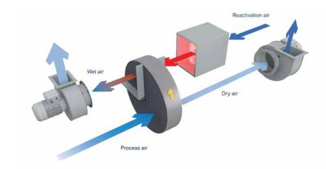
Humiscope are leaders in dehumidification technology. We custom design desiccant dehumidifiers to the precise specifications required for your low dew point application.
